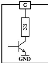
Programmable outputs C1, C2, C3 and C4 are used to connect remotely controlled devices.
