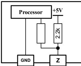
Inputs Z1-Z14 are used to connect sensors of protected zones or temperature sensors KTY81-110 (PHILIPS).
