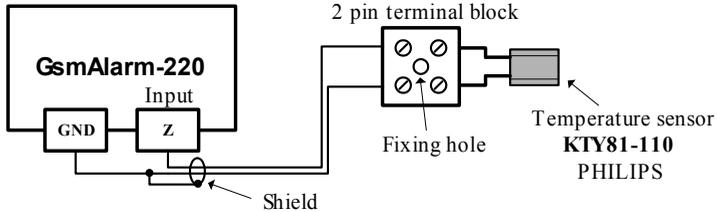
In order to minimise influence of external interferences and measurement error, it is recommended to use shielded twisted pair cable 0.5 mm<sup>2</sup>.
