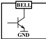
The BELL output is used to connect audio siren or extra-commutated device.
